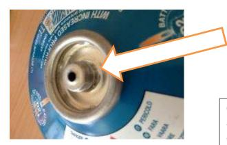
The fitting must have a thread. The canister must screw on to the gas burner.
